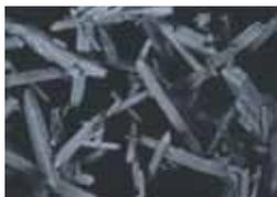
Improved Paste and 4BS (Tetra Basic lead sulphate) application to longer life cycle and capacity maximization
